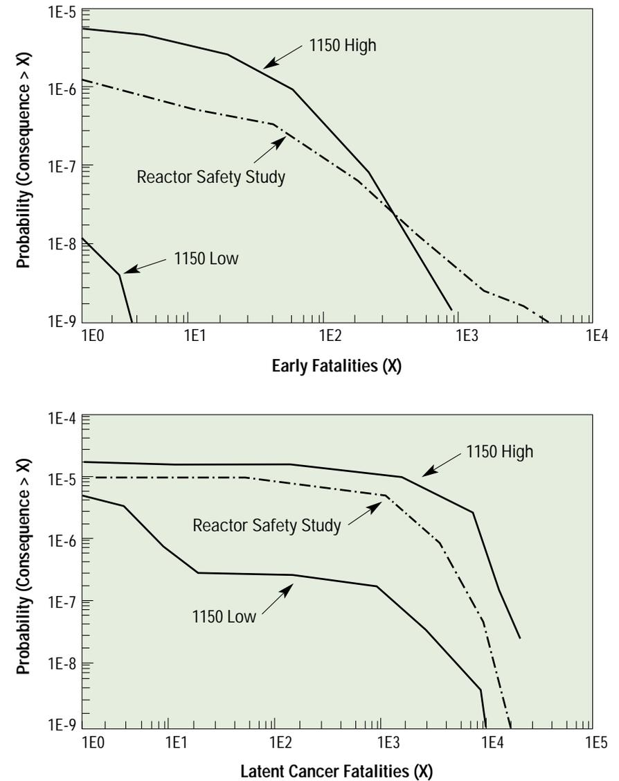
Figure 3 Comparison of the cumulative frequency of occurrence damage function between NUREG-1150 and RSS (Wash-1400)
